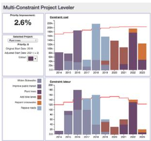
A software tool for scheduling projects with multiple resource constraints was developed. A variety of constraint programming, integer programming and local search techniques were applied to guide the user to optimal or near-optimal solutions. A mixed-initiative approach was used to allow for collaboration between the user and the software through a novel interactive visualization of the optimization problem.
