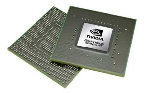
Graphic Processing Units (GPUs) are co-processors that can simultaneously perform a simple computation on multiple batches of data. In contrast, a CPU can perform more complex computations but not in parallel. This project has extended Threading Building Blocks (open source C++ library) to run computational tasks on the CPU or GPU.
