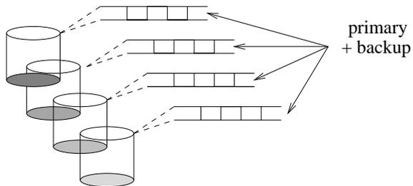
Figure 4: **Mirroring Reservation.** For each disk, there is a separate vector indexed by round number that accumulates the total estimated access time for retrieving primary and backup data in each round.
