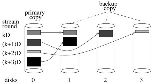
Figure 2: **Deterministic Replica Placement.** Data of a media file stored consecutively on disk 0 and retrieved during different playback rounds are replicated round-robin across the other disks. The primary data of the other disks are replicated in a similar way.
