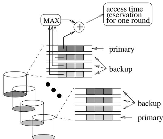
Figure 5: **Minimum Reservation.** For each disk, we maintain  $D$  separate vectors indexed by round number. One of them accumulates access delays for retrieving primary data. The remaining  $D - 1$  vectors accumulate access delays for retrieving backup replicas that correspond to primary data stored on each of the other  $D - 1$  disks. In each round, the sum of the primary data access time and the maximum of the backup data access times is reserved on each disk.
