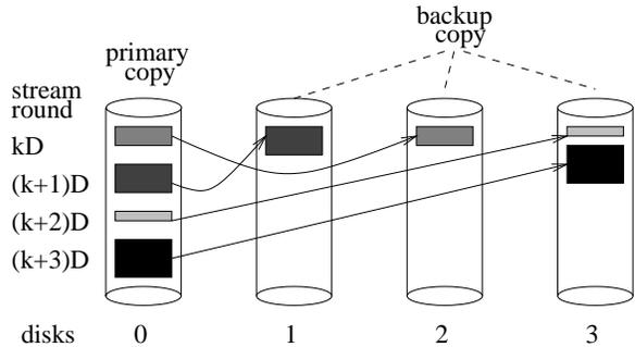
Figure 3: **Random Replica Placement.** Data of a media file stored consecutively on disk 0 and retrieved during different playback rounds are replicated on randomly chosen disks 1 to 3. The primary data copies of disks 1 to 3 are replicated in a similar way.
