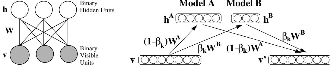
Figure 1: **Left:** Restricted Boltzmann machine. The top layer represents a vector of stochastic binary units  $\mathbf{h}$  and the bottom layer represents a vector of stochastic binary visible variables  $\mathbf{v}$ . **Right:** The Gibbs transition operator  $T_k(\mathbf{v}'; \mathbf{v})$  leaves  $p_k(\mathbf{v})$  invariant when estimating the ratio of partition functions  $Z_B/Z_A$ .
