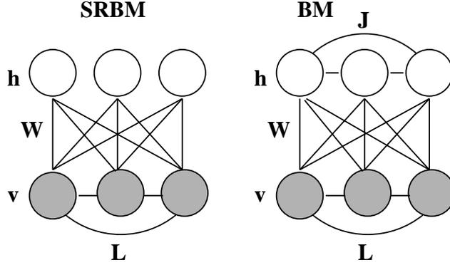
Figure 2: **Left:** Semi-restricted Boltzmann machine. The visible units form a fully or partially connected conditional MRF, with hidden units determining the biases of the visible units. **Right:** Boltzmann Machine with both visible-to-visible and hidden-to-hidden connections.
