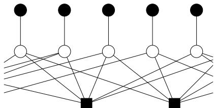
Notice that each codeword bit connects to three parity checks — corresponding to the three 1s in each column of  $H$ . Each parity check connects to six codeword bits.
