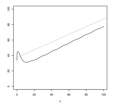
The constant of proportionality seems to be 0.5 (grey line has that slope). But if this is the time for a program to run, that constant will vary from computer to computer.
