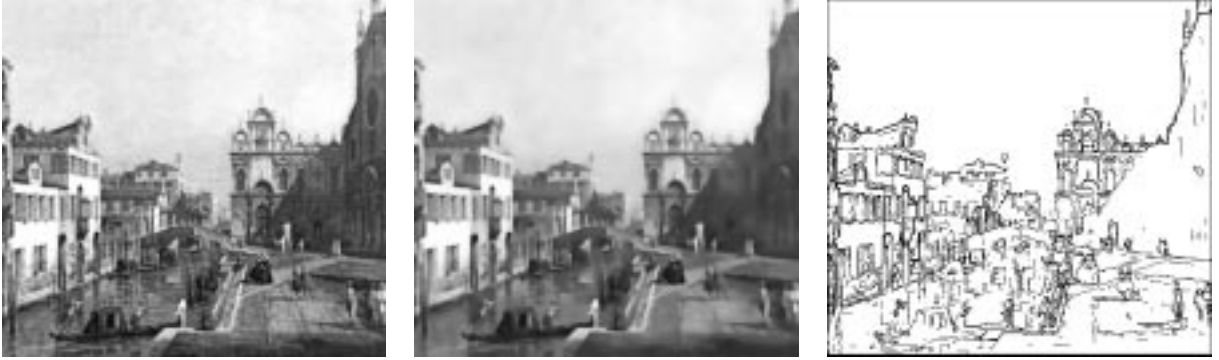
Figure 4: (Left) Input Image. (Middle) Regularization result using a robust Lorentzian error norm for the smoothness constraint. (Right) Edges obtained at pixels which are indicated to be outliers according to the Lorentzian error norm.
