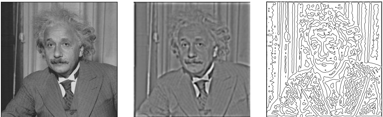
Figure 3: From left to right is the original AI, a band-pass filtered version of AI, and the zero-crossings of the filtered image. This impulse response is defined by the difference of two low-pass filters.
