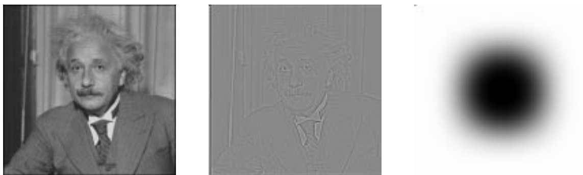
Figure 4: From left to right is the original AI, a high-pass filtered version of AI, and the amplitude spectrum of the filter. This impulse response is defined by \delta[n] - h[n, m] where h[n, m] is the separable blurring kernel used in the previous figure.
