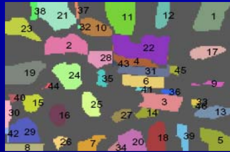
Seed regions found through spectral clustering. Combinations of these are used as source and sink regions for S-T MinCut
