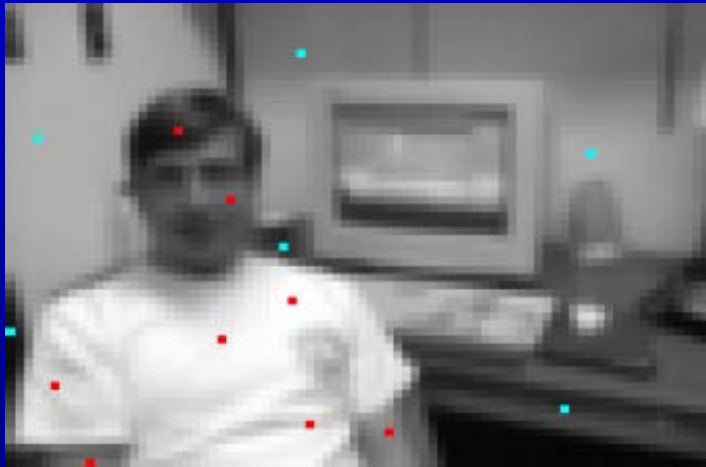
User-selected pixels connected to S (red) and pixels connected to T (cyan)
