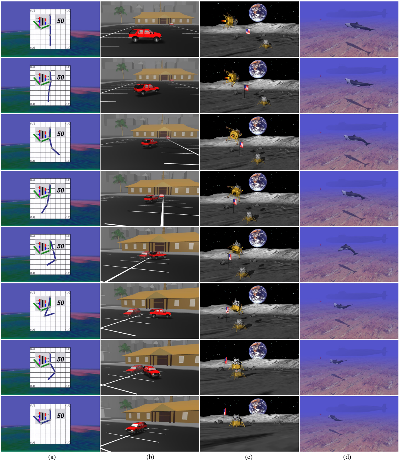
Figure 13: Results of applying the control learning algorithm to four different NeuroAnimators. (a) The 3-link pendulum NeuroAnimator in purple must reach the state indicated in green with zero final velocity. (b) The truck NeuroAnimator learning to park in the position and orientation of the translucent vehicle in the background. (c) The lunar lander NeuroAnimator learning to land with low descent velocity in the position and orientation of the translucent vehicle on the surface. (d) The dolphin NeuroAnimator learning to swim. The objective of locomoting as far forward as possible produces a natural, periodic swimming pattern.
