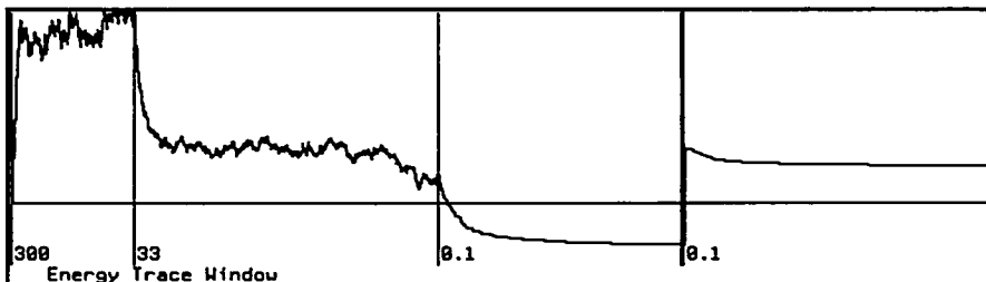
Figure 12. A graph of the energy level as the network follows the temperature schedule of Figure 11. Thin vertical divisions mark temperature changes, with the new temperature shown at the bottom of the graph. A thick division marks the point where thresholds are raised in the rebiasing step.
