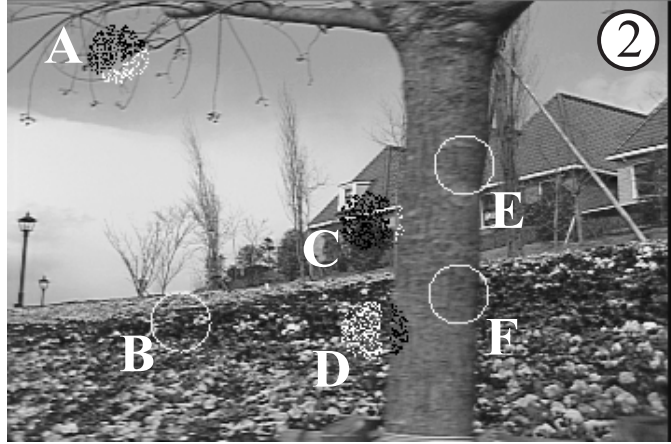
Figure 7 Flower Garden results at frame 2 are shown, with the most likely models overlaid on the image. Translational models are shown as empty circles (as in region B ). Motion boundaries are shown as filled disks (as in region D ). The white and black dots, respectively, lie on the foreground and background sides of the model. The position and orientation of the boundaries are depicted by the edges between the white and black sides.
