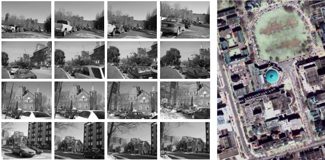
Figure 3: Left: Four segments of an image sequence from the training dataset. The camera pose of consecutive images changes slowly so that two neighboring images share some features. Right: The satellite map of the whole region for taking image data, overlapped with the trajectory of the camera. (©Google Maps, Imagery ©DigitalGlobe).
