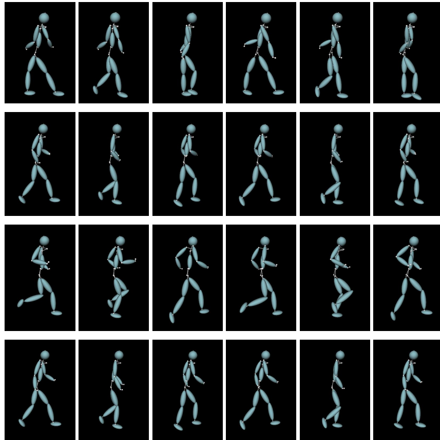
Figure 4.11: Sampling the first two components of a multi-activity database compose of walking and running motions can produce physically impossible motions. The coefficients of the motions depicted in this figure are shown in Fig. 4.10. Top row: Physically impossible motion. The input motion space compose of walking and running is not convex. Middle row: Physically possible motion close to a walking. Bottom row: Motion close to a running. As the convexity of the input space is assumed when doing PCA, and it may not be the case, the resulting motion as a combination of principal directions can be physically impossible.
