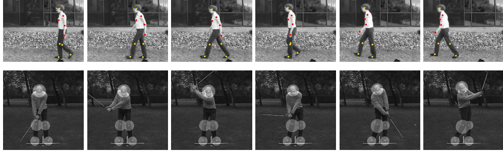
Figure 4.12: 2D Tracking using the WSL tracker. Top row: Tracking the chest, knees, head, ankles and visible arm. The tracked upper body joints are shown in red, with the head and tracked lower joints points shown in yellow. Bottom row: Regions used for tracking the ankles, knees, and head are shown.
