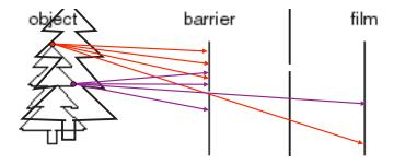
Add a barrier to block off most of the rays
