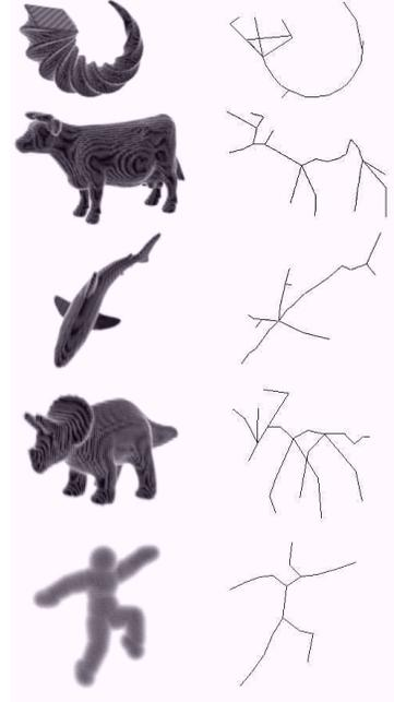
**Figure 3. Sample skeletal graphs:In the left column, different volumes are shown. In the right are the resulting skeletal graphs.**
