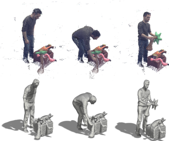
Figure 5. Temporal consistency pipeline. Top: Point cloud visualization, notice flying pixels and holes. Bottom: temporally reconstructed meshes.
