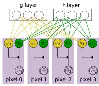
Figure 1. Graphical model of the Robust Boltzmann Machine. Filled triangles indicate gating of the connection between  $v_i$  and  $\tilde{v}_i$  by  $s_i$ . The yellow connections are the weights of the RBM while the green connections are the weights of the GRBM. Each pixel is modeled by three random variables:  $v_i$ ,  $\tilde{v}_i$  and  $s_i$ . Best viewed in color
