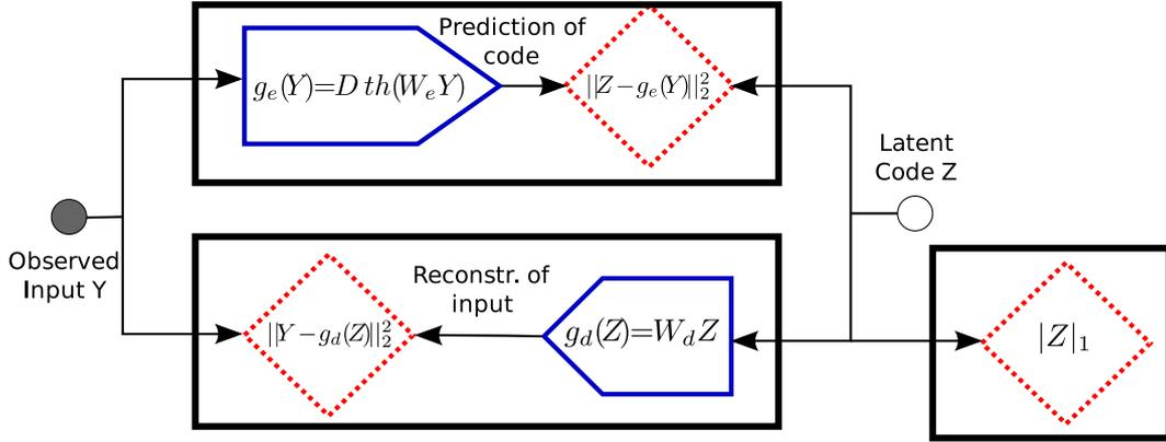
Figure 3.1: Graphical representation of PSD algorithm learning sparse representations.
