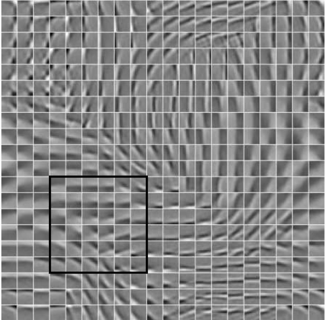
Figure 4.5: Topographic map of feature detectors learned from natural image patches of size 12x12 pixels by optimizing the loss in eq. 4.3. There are 400 filters that are organized in 6x6 neighborhoods. Adjacent neighborhoods overlap by 4 pixels both horizontally and vertically. Notice the smooth variation within a given neighborhood and also the circular boundary conditions.
