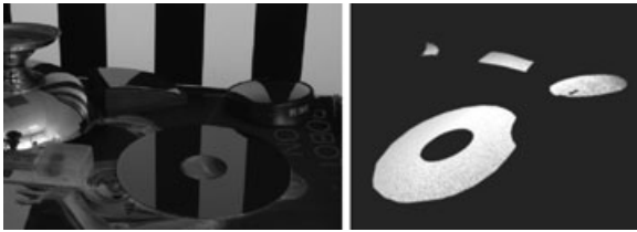
Figure 6: Shape reconstruction of specular objects using direct ray measurements. An input photograph with three curved and one planar specular object (left panel) and reconstruction result seen from a different view-point (right panel). The large object to the left has only been partially reconstructed due to missing pattern information. Image courtesy of Thomas Bonfort, Peter Sturm and Pau Gargallo [BSG06].
