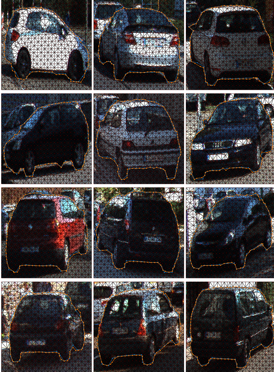
Fig. 7: Deformed Grid: We show examples of predicted grids on KITTI. Blue line is CurveGCN's prediction and orange line is searched minimal energy path.
