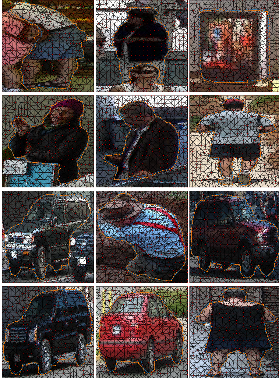
Fig. 6: Deformed Grid: We show examples of predicted grids on the ADE dataset. Blue line is CurveGCN’s prediction and orange line is searched minimal energy path.
