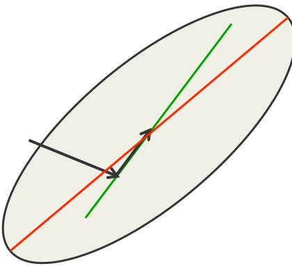
The gradient in the direction of the first step is zero at all points on the green line.
