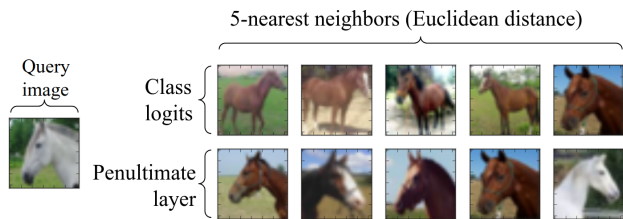
Figure 2. Finding the nearest neighbor in a network trained on CIFAR-10. Query is a close-up on a horse’s head. If the nearest neighbor is calculated in the “class” logits layer, we find examples from the same class (horse), but the semantically similar image with a close-up head is only the 5 th nearest-neighbor. If distance is calculated in the penultimate layer, all nearest neighbors are semantically similar to the query. This shows that some semantic information is lost in the “class” logits and distillation can benefit from using more information.
