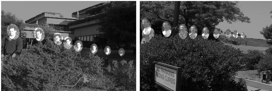
Fig. 7. Tracking with partial occlusion along with variable lighting, appearance, and size. The camera was stationary and the sequences are each roughly 250 frames. The highlighted target region for selected frames is superimposed on the last frame.
