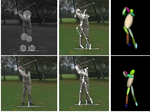
Figure 6: Tracking using only joint constraints vs using the complete objective function. Top: Using only joint constraints the problem is under-constrained and a multiple set of solutions are possible. Bottom: The set of solutions is reduced using correspondences.
