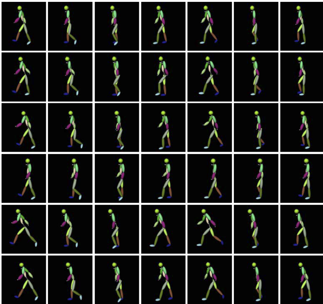
Fig. 3. The top row shows equispaced poses of the mean walk. The next five rows illustrate the influence of the first five eigen-motions. The second row shows a linear combination of the mean walk and the first eigen-motion, \theta_0 + 0.7\theta_1 . Similarly, the third row depicts \theta_0 + 0.7\theta_2 to show the influence of the second eigen-motion, and so on for the remaining three rows.
