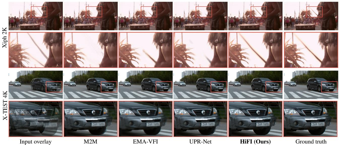
Figure 5: **Qualitative examples for public datasets.** Our method performs well even in cases of large motion and complex textures such as a thin object on the top and the plate number at the bottom.
