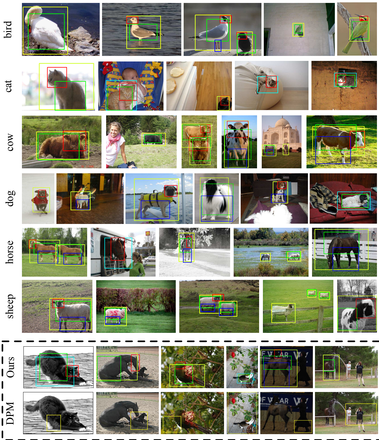
Figure 5. Our method provides a richer representation for the deformable objects and improves detection results on difficult examples. The red, green and blue boxes correspond to head, torso and legs, respectively. The holistic object boxes are shown in yellow, and the cyan boxes correspond to the generated holistic object bounding box (note that we should generate a bounding box for patterns whose holistic object node is switched off). In the dashed box, we also show examples of animals correctly localized by our method but missed by DPM.
