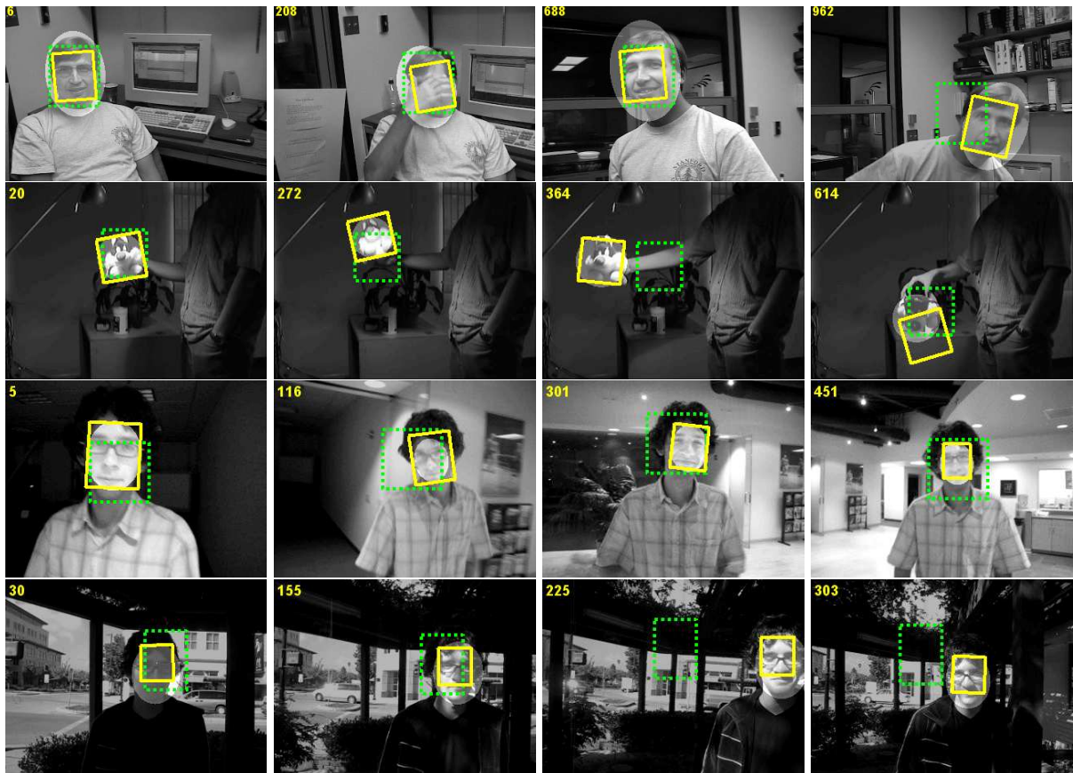
Figure 2.10: A comparison of our tracker (indicated with a yellow box) with the WSL (Jepson et al., 2003) (shown in highlighted ellipse) and the Mean Shift (Comaniciu et al., 2003) (depicted by a green dashed box) on four video sequences.
