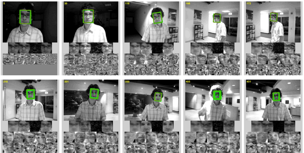
Figure 2.6: A person moves from a dark to a bright area, undergoing large lighting and pose changes. The images in the second row show the current sample mean, tracked region, reconstructed image, and the reconstruction error respectively. The third and fourth rows show the top 10 principal eigenvectors.
